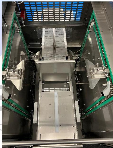
Exact turning unit together with pusherplate provides a stable stack.
