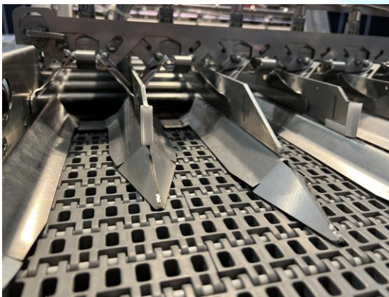
Moving infeed guides. Easy adjustable gates for different egg-sizes.
